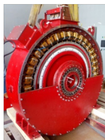
Traction motor generator on permanent magnets 400 kW, 130 rpm
