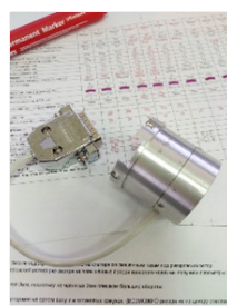
Synchronous micromotor for drive of cryogenic system 25W, 4000 rpm
